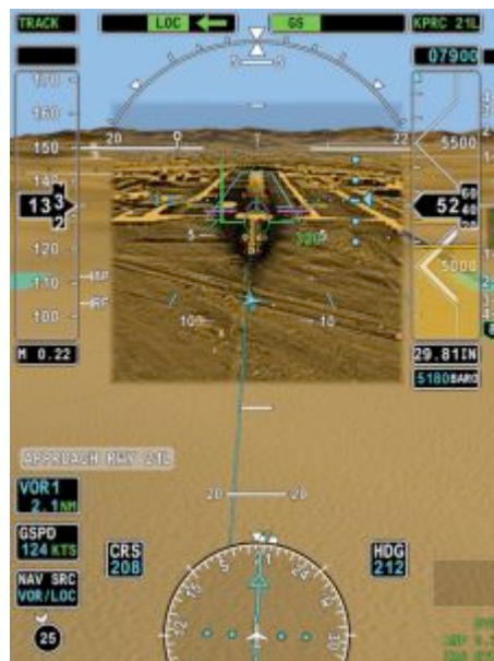
Honeywell's synthetic vision technology is blended with real-world data in this enhanced vision display showing a runway approach.
