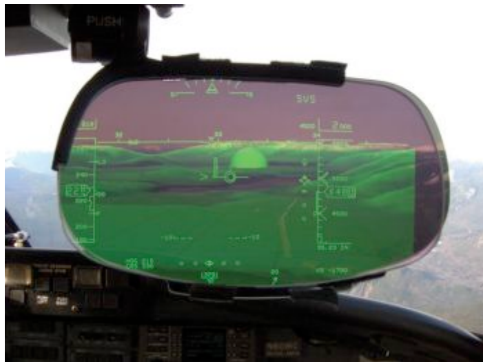
Synthetic vision technology from Rockwell Collins is viewed through a heads-up display (HUD).
